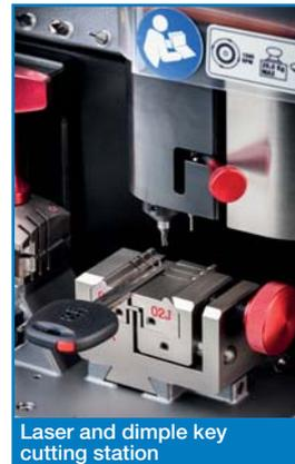
Laser and dimple key cutting station
