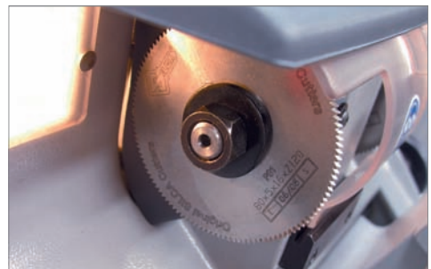
Prismatic cutter made of HSS
